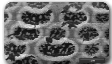
builds in longevity. Another advantage is the excellent, permanent optical contrast that comes from making a physical mark. The difference in optical quality between the pit, where there is no material, and the areas adjacent to the pit, where the material remains, provides a definite advantage in retention of data and in ease of reading the disc decades into the future.
