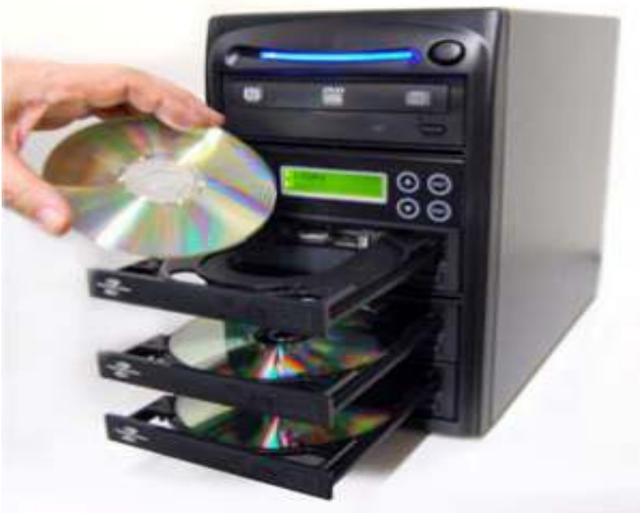
Go to menu "**11. LightScribe**" by pressing UP or DOWN buttons. Then press "ENT" key into menu "**Print**" and press "ENT" key to start the label printing process last.
