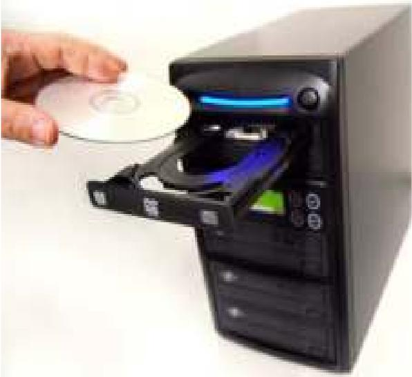
Place a recordable LightScribe disc into the target LightScribe recorder with the **label side facing down**.
